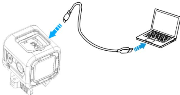
Connect the camera to your computer using the included C-type USB cable.
